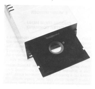
The blank diskettes you are copying onto should be inserted with the label side up, as usual.
